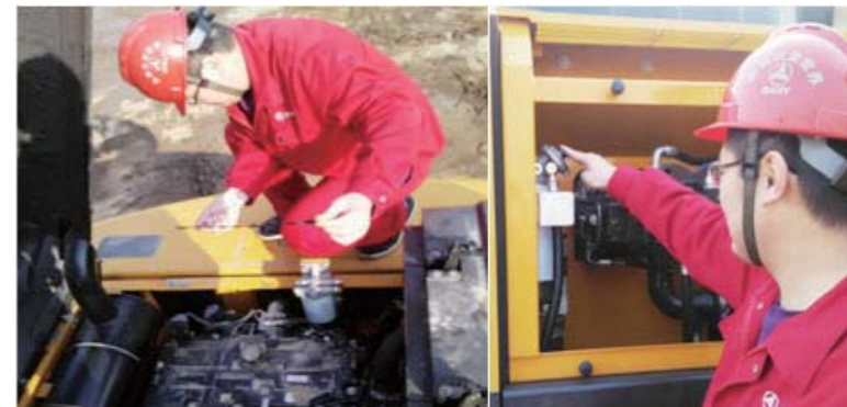
Inspect the situation of engine oil
